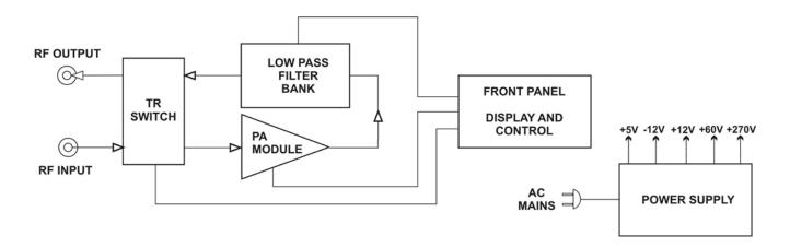
When the KPA500 is in operating (OPER) mode, RF is routed by the transmit-receive (TR) switch to the power amplifier (PA) module where it is amplified by a pair of VRF2933 FETs.
