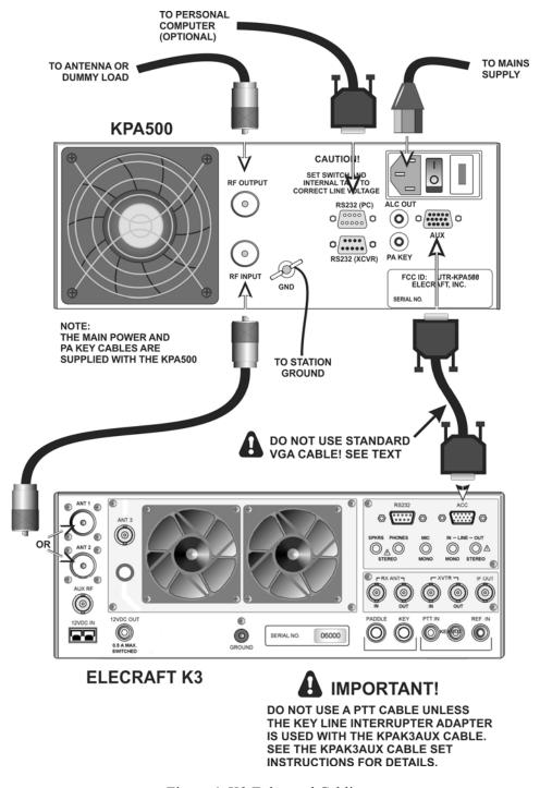
Figure 4. K3 Enhanced Cabling.
