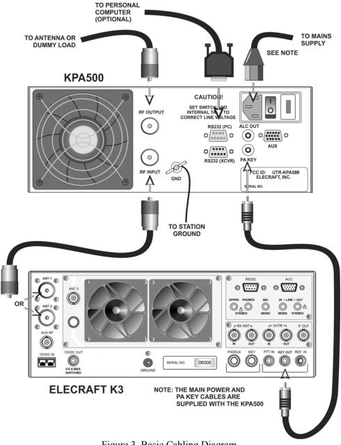
Figure 3. Basic Cabling Diagram.
